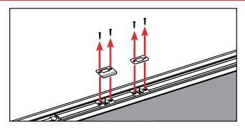
a. Unscrew the deadbolt plate and the strike plate and remove. Keep the screws with the respective plates to reinstall correctly.
