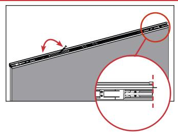
d. Lock the flip lever to ensure the bolt is actively engaged. Ensure that when the flip lever is in the unlocked position, the end of the bolt is either flush with the end of the astragal body or slightly inset.
