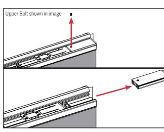
c. Unscrew and remove the bolt sleeves off the upper and lower bolts to reveal additional securing screws. (Only upper bolt shown in image)
