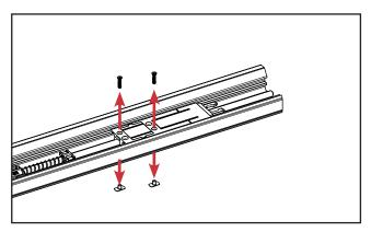
a. Loosen and remove screws that hold the bolt in place. Remove the T-nuts that hold the screws on the back side of the astragal.
