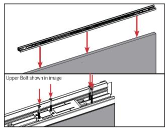
c. Return astragal to the door panel and reinstall the screws back through the astragal into the door panel, starting with the screws under the bolt sleeve.
