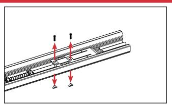
b. Screw the shoot bolt in place using the T-nuts and smaller screws in the smaller screw holes.
