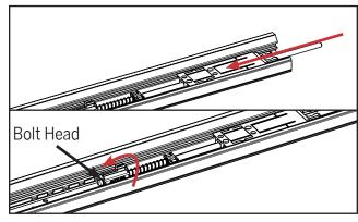
a. Slide the new bolt assembly into the astragal body. Rotate the bolt head into the exact position from which the previous bolt was removed.
