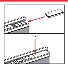
a. Slide the bolt sleeve in and screw back in place.
