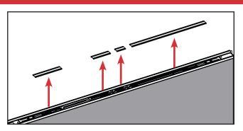
b. Remove the trim strip along the entire astragal body to expose the screws that secure the astragal on to the door panel. Note where the 4 pieces of the strip belong, as you will have to return them to the exact position.
