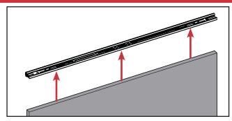
f. Pry the astragal off the door panel. **We recommend you use help to do this.** Lay the removed astragal body on a flat work surface.
