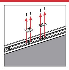
c. Once both retainers are in the astragal, screw on the strike plate and the deadbolt plate, using your best judgment for horizontal alignment.
