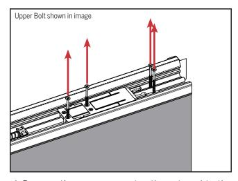
d. Remove the screws securing the astragal to the door panel. The astragal may still be attached to the panel due to the presence of a strong tape on the back adhering it to the panel.
