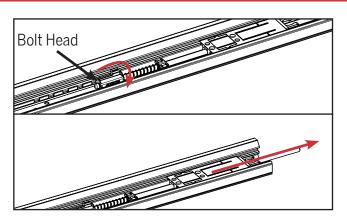
b. Rotate the bolt head out of the drive rod and then slide the bolt assembly out of the astragal body.
