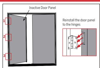
Reinstall the inactive door panel by screwing the door panel back to the hinges.
