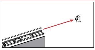
e. If necessary, remove the trim caps on the top and bottom of the door to expose a channel to grasp the astragal.
