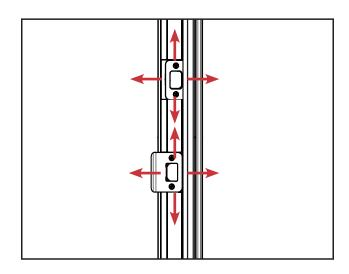
b. Adjust the location of the plate if necessary by loosening the screws and sliding the plate horizontally.
