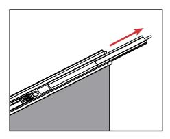
a. Slide out the upper flush bolt from the astragal body.
