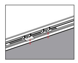
a. Use the marks in step 2b to align the center lines of the strike and deadbolt plates and retainers.
