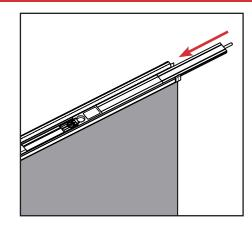
c. Slide the upper flush bolt back into the astragal body.
