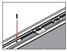
f. Secure the strike support with the 1-5/8" screw provided.
