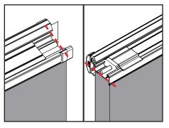
d. Position the upper and lower flush bolts so the pins align with the end of the astragal body.
