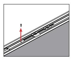
e. Remove the screw from the existing strike support. Slide the strike support out of the body.
