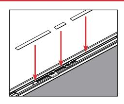
c. Reinstall the strike support trim into the new strike support.
