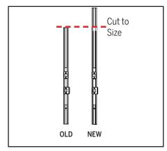
a. Position the replacement strike support next to the old strike support. Cut the replacement strike support to match the length of the old strike support.
