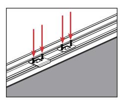
b. Tighten the screws into the strike and deadbolt plates to secure them in their location. Wipe away the pencil marks.
