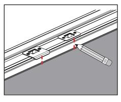
b. Using a pencil, mark the center line of the plate opening(s) on the edge of the astragal body.
