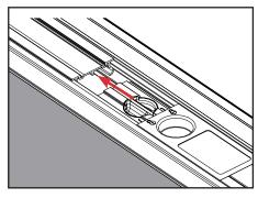
e. Position the strike support so the inner ends of each bolt slide under the strike support.
