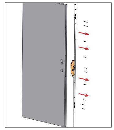
**a.** Remove the screws securing the lock to the door panel. Remove the lock from the door panel and discard.
