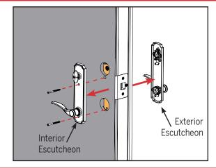
Remove the screws securing the handset from the interior escutcheon. Make sure to hold the exterior escutcheon as the screws are being removed to prevent damage. Set aside the handset along with all of the internal components.
