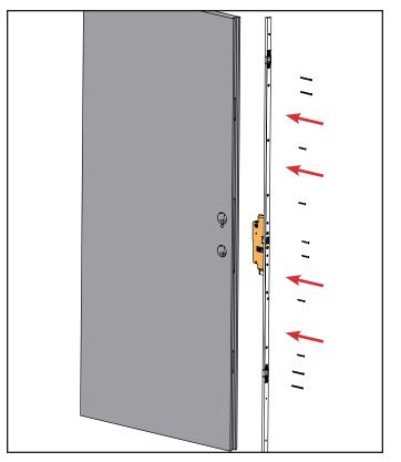
**b.** Insert the new 3020 lock into the pocket in the door from which the old lock was removed. Secure the lock in place with the screws provided.
