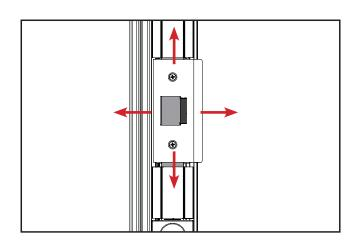
b. Adjust the location of the plates if necessary by loosening the screws and sliding the plate horizontally.
