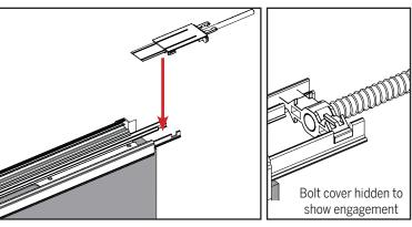
a. Return the shoot bolt so its engagement head notches securely into the grooves on the metal driver rods.
