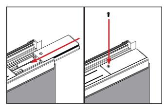
a. Return the bolt sleeves to the top and bottom of the astragal and secure them with the screws previously removed.
