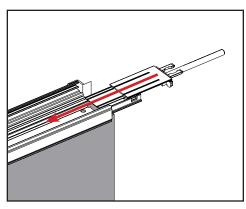
b. Slide the metal driver rods back into the astragal body, along with the shoot bolt.
