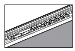
c. Replace the spine assembly in the exact location it was removed from. Align the bolt engagement head into the metal driver rods and rotate the spine assembly into the astragal body.
