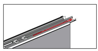
Remove the old strike retainer to be replaced from the astragal body.
