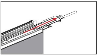
b. Slide out the metal driver rods from the astragal body, moving the upper shoot bolt with it.
