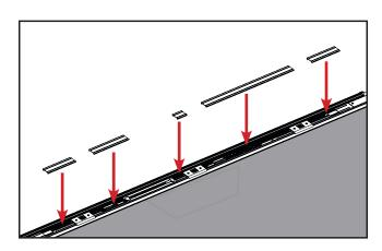
b. Return the trim strip on the door in the same locations that they originally were. Use this to guide adjust where the strike retainer will sit.
