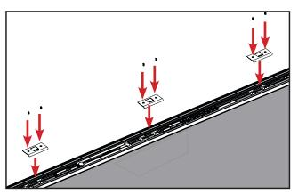
Return the strike plates on the retainers and screw back in place.
