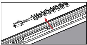
a. Rotate the engagement head and spine assembly in order to remove them from the metal driver rods.
