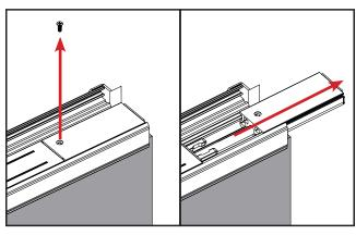
c. Unscrew and remove the bolt sleeves off the top and bottom bolts to reveal additional securing screws.
