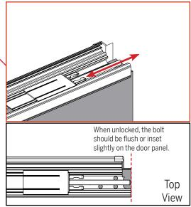
d. Check operation of the flip lever assembly and shoot bolts. When the flip lever is in the unlocked position, the end of the bolt must be either flush with the astragal body or slightly inset. When the flip lever is in the locked position, ensure the entire spine assembly and shoot bolt extend together.
