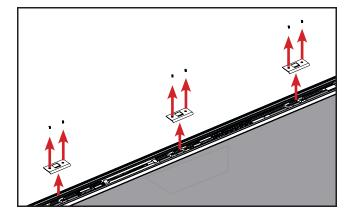
b. Unscrew the strike plates and remove.
