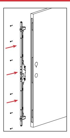
Place the new lock face out into the channel. Ensure the lock faceplate is flush with the panel. Screw the lock in using the screws provided.
