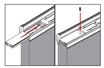
h. Return the bolt sleeves to the top and bottom of the astragal and secure them with the screws previously removed.
