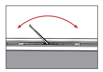
i. Operate the flip lever to ensure the bolt is actively engaged. Ensure that when the flip lever is in the unlocked position, the end of the bolt is either flush with the end of the astragal body or slightly inset.
