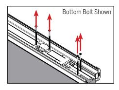
e. Remove the screws securing the astragal to the door panel. The astragal may still be attached to the panel due to the presence of a strong tape adhering it to the panel.
