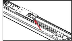
Remove the deadbolt actuator by rotating the engagement head out of the channel and lifting.
