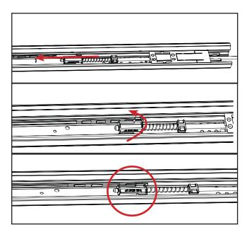
a. Return the shoot bolt into the astragal in the exact position that you removed it from by angling and placing the white head into the channel.
