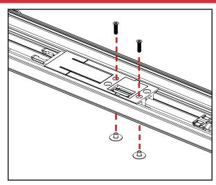
a. Loosen and remove screws that hold the bolt in place. T-nuts hold the screws on the back side of the astragal. Remove these and set aside.
