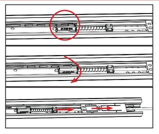
b. Slide the shoot bolt out by first angling the white head out of the channel and then sliding out of the astragal body.
