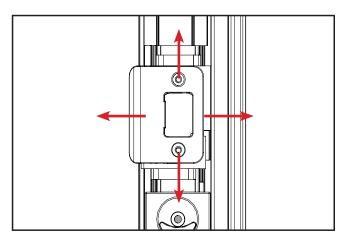
b. Loosen screws and adjust the plate and retainer location, if necessary.
