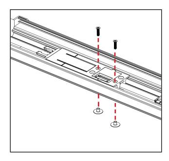
b. Return the top shoot bolt and screw in place using the T-nuts and smaller screws in the smaller screw holes.
