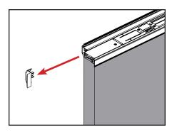
f. If still attached, remove the trim cap on the top of the door exposing a channel to grasp the astragal.
