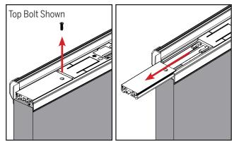
c. Unscrew and remove the bolt sleeves off the top and bottom bolts to reveal additional securing screws.
