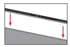
g. Return the astragal to the door panel and screw into place, returning all of the screws removed previously from the door panel.
