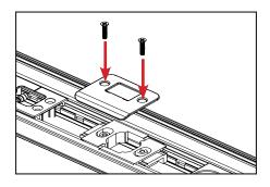
e. Return strike plate onto the retainer and screw back in place.
