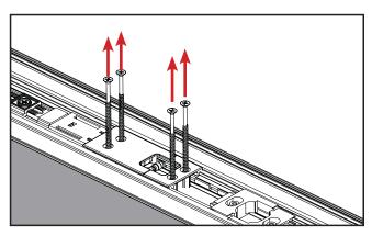
d. Remove the screws securing the deadbolt actuator through to the door panel.
