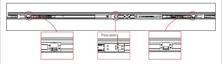
d. Press down on the actuator to ensure it engages the top and bottom lock pawls. Adjust the engagement head if necessary.
