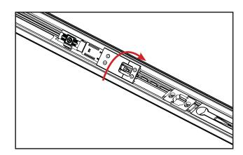
c. Return the actuator to its exact location on the operating channels and screw into place.
