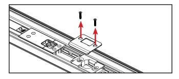
b. Unscrew the strike plate and remove.
