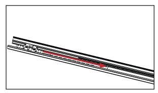
Slide the strike retainer out of the astragal, and replace by sliding a new one in its place.
