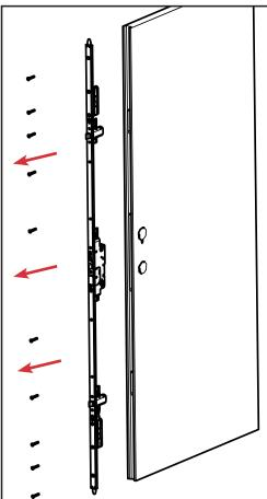
Loosen the screws that secure the lock on the panel and remove the existing lock. Clear out any debris that may be in the exposed channel. You do <u>not</u> need to remove the torxhead screws.
