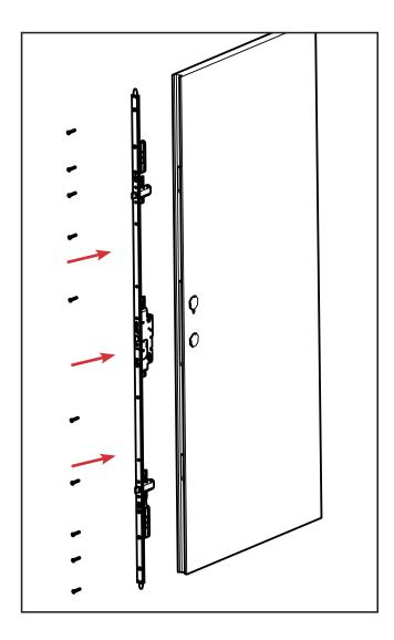
Place the new lock face out into the channel. Ensure the lock faceplate is flush with the panel. Screw the lock in using the screws provided.
