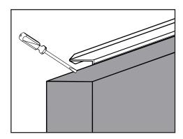
a. Remove the old DoorTop from the door panel. Use a flathead screwdriver to pry the end of the DoorTop up.
