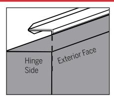
a. Orient the DoorTop with the door panel as shown above. Align the DoorTop flush to the edge of the hinge side.
