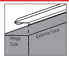
b. Align the end of the DoorTop seal flush to the edge of the hinge side along the outside of the door panel.
