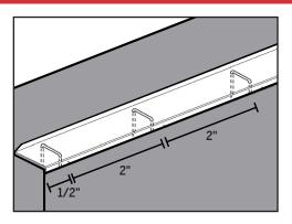
b. Attach the DoorTop to the top of the door panel using 1/2" x 1/2" staples. Position staples 1/2" from the end of the doortop and space them 2-4" apart. Close the door to confirm proper installation.
