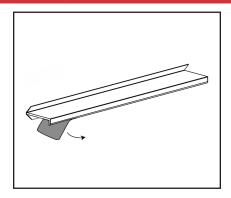
a. Remove the backing strip from attachment tape on underside of DoorTop
