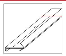
b. Measure and mark the same width (X) on the DoorTop, measuring from one end. Cut the DoorTop along this line.
