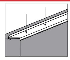
c. Press the DoorTop firmly onto the panel along the entire length. Close the door to confirm proper installation.
