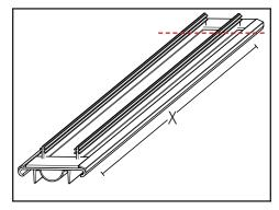
b. Measure and mark the same width (X) on the door bottom, measuring from one end. Cut the door bottom at this line.
