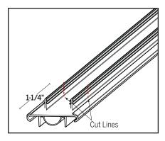
b. If the notch is less than 1-1/4", renotch the kerf legs. Measure 1-1/4" from the end of the door bottom and make a cut into the kerf legs.
