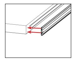
b. Using hand pressure (or a rubber mallet), fully insert the door bottom kerf legs into the panel slots, ensuring ends remain flush.
