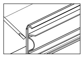
a. Remove the old door bottom from the door panel. Use a flathead screwdriver to pry the end of the door bottom off the panel.
