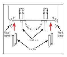
c. Complete insertion by moving along the length of the door bottom. Secure each end with a 1/2" x 1/2" light gauge staple.
