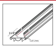
c. Cut the kerf legs, where they meet the door bottom until they are removed. Be sure to cut the kerf legs as close to the door bottom as possible to ensure a flat surface.
