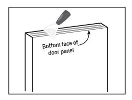
b. Remove any old residue or staples from the door panel's bottom face, using a putty knife or similar tool.
