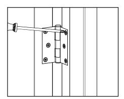
a. Open the door and locate the hinges. Using a Phillips screwdriver or drill remove the screws from the hinge plate on the jamb.
