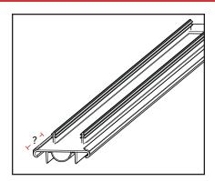
a. Measuring from the cut end of the door bottom, determine if the notch is greater or less than 1-1/4". If the notch is greater than 1-1/4", move to step 5.
