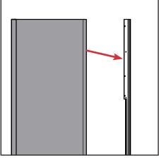
b. Starting at one end, pry the flange from the door panel, working along the length.
