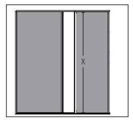
a. Measure the length of the active door panel (X). If the door bottom is attached, do not include this in the measurement.
