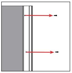
a. Remove the screws along the entire length of the flange.
