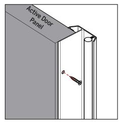
b. Insert the screws through the predrilled holes to secure the flange snug against the face of the active door.
