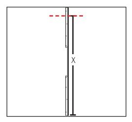
b. Cut the replacement flange to the same length as the door panel. Make the cut from the top end.
