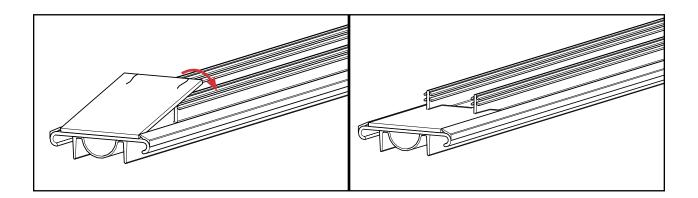
**C:** Install the new door bottom by inserting the kerf legs into the panel slots and secure each end with staples. Repeat for the other door panel.
