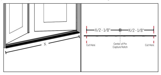
**4C:** Return the two spring loaded bases on each end of the cut sill cap.
