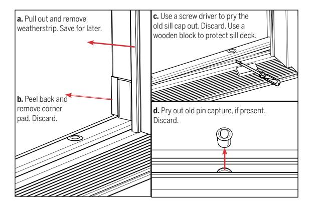
Step 2: Remove the door panels from the frame.
