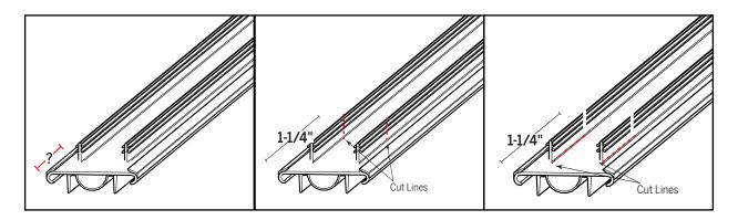
**B:** Apply the door bottom gasket, ensuring the solid edge is flush with the cut edge of the door bottom.
