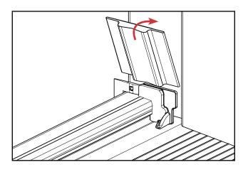
Remove paper backing and align bottom of corner pad flush against the top of the stiffener.
