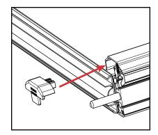
Align the trim cap with astragal body and insert into the bottom of the astragal.
