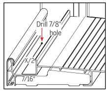
Drill hole for pin capture with a diameter of 7/8".
