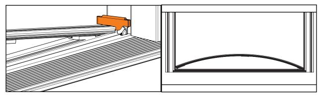
Align edge of cap with mull stiffener on one end.
