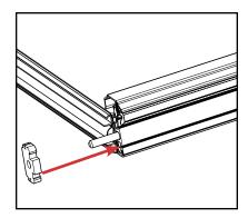
Engage flush bolt and align hole on the astragal bottom gasket with the bolt. Press against the panel.
