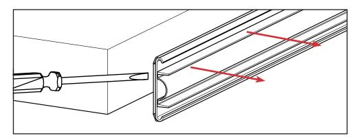
On the inactive door panel, remove these components from the astragal:
