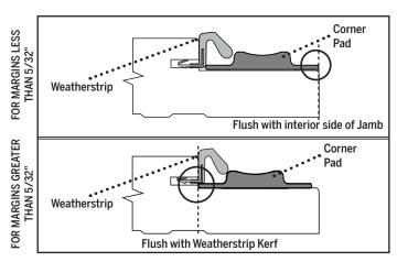
Align with weatherstrip and jamb based on strike margins. Press corner pad firmly against jamb and confirm the door operates properly. The sill cap should move up and down as the door opens and closes. Repeat on other side.
