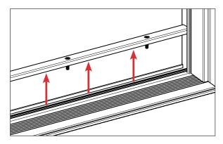
**b.** Pull the sill cap out of the channel and set aside.
