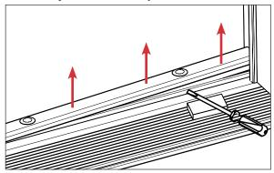
a. Pull up on the old sill cap using a flathead screwdriver to loosen it from the sill.
