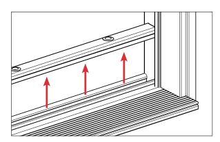
**b.** Pull sill cap out of channel and set aside.
