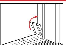
**c.** Align the bottom of the corner pad against the top of the sill cap.
