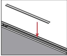
b. Reinstall the trim strip into the astragal body, helping to align the deadbolt and strike retainers.
