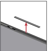
b. Remove the trim above the **deadbolt** plate if removing the deadbolt retainer or remove the trim below the **strike** plate if removing the strike retainer.
