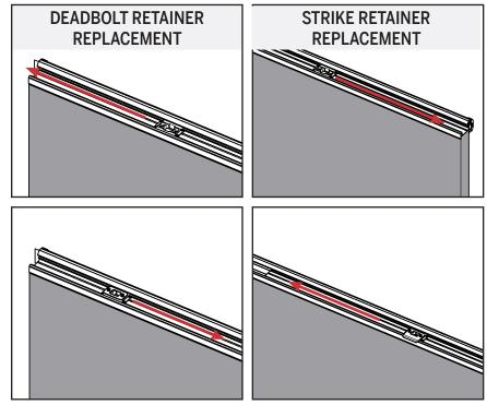
a. Slide the old deadbolt or strike retainer out of the astragal body and slide the new deadbolt or strike retainer into the astragal body.
