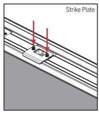
Tighten the deadbolt or strike plate in place, using best judgment for horizontal alignment.
