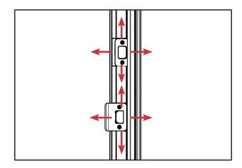
b. Adjust the location of the plate if necessary by loosening the screws and sliding the plate horizontally.
