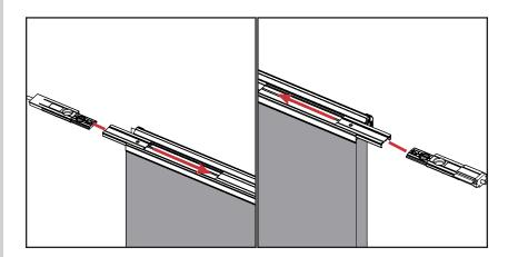
a. Slide the locking bracket (if present) and flush bolt back into the astragal body. The flush bolt should be flush with the end of the astragal body.
