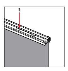
b. If the locking bracket is present, reinstall the screw back into the bracket.
