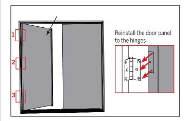
a. Reinstall the inactive door panel by screwing the door panel back to the hinges.
