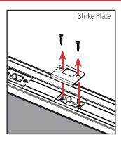
a. Remove the screws holding the deadbolt plate if you are removing the deadbolt retainer or remove the screws holding the strike plate if you are removing the strike retainer.
