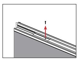
b. If present, remove the screw securing the strike support and remove the strike support.
