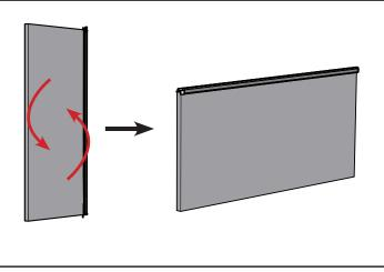
a. Remove the inactive door panel by unscrewing the door from the hinges.
