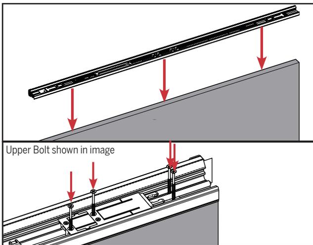
c. Return astragal to the door panel and reinstall the screws back through the astragal into the door panel, starting with the screws under the bolt sleeve.
