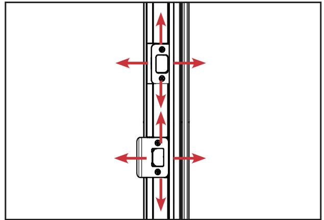
b. Adjust the location of the plate if necessary by loosening the screws and sliding the plate horizontally.
