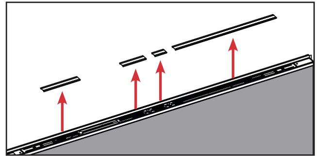
b. Remove the trim strip along the entire astragal body to expose the screws that secure the astragal on to the door panel. Note where the 4 pieces of the strip belong, as you will have to return them to the exact position.
