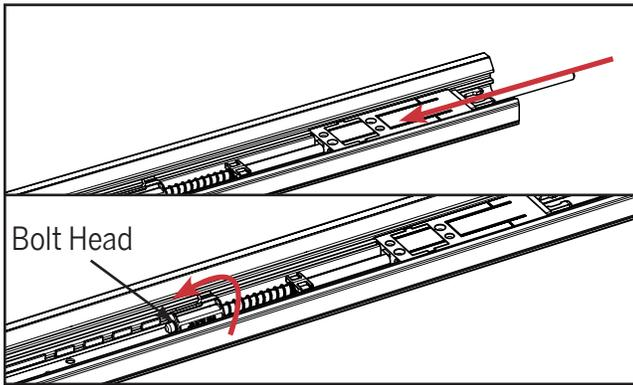
a. Slide the bolt assembly into the astragal body. Rotate the bolt head into the exact position from which the previous bolt was removed.
