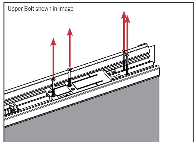
d. Remove the screws securing the astragal to the door panel. The astragal may still be attached to the panel due to the presence of a strong tape on the back adhering it to the panel.
