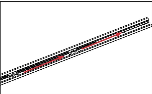
a. Slide the strike retainer out of the astragal. If you are replacing the deadbolt retainer, slide this out of the astragal body as well.
