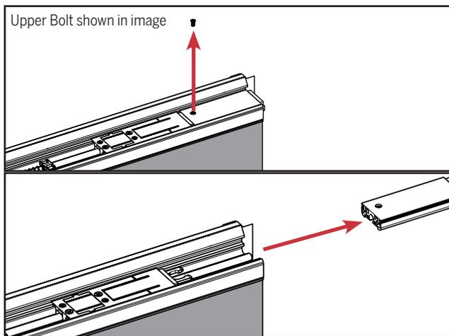
c. Unscrew and remove the bolt sleeves off the upper and lower bolts to reveal additional securing screws. (Only upper bolt shown in image)
