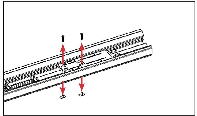
b. Screw the shoot bolt in place using the T-nuts and smaller screws in the smaller screw holes.
