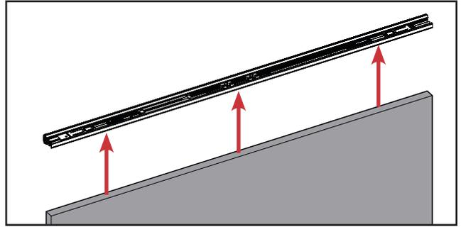
f. Pry the astragal off the door panel. **We recommend you use help to do this.** Lay the removed astragal body on a flat work surface.
