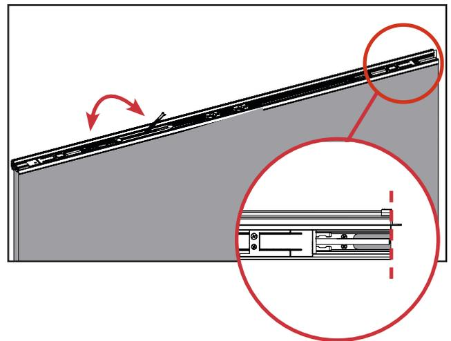
d. Lock the flip lever to ensure the bolt is actively engaged. Ensure that when the flip lever is in the unlocked position, the end of the bolt is either flush with the end of the astragal body or slightly inset.
