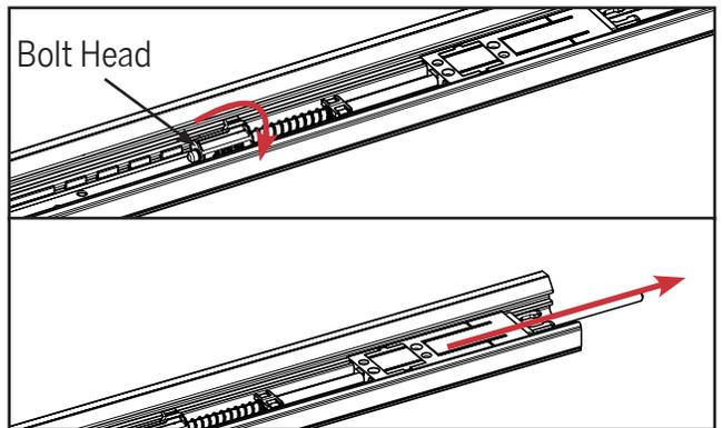
b. Rotate the bolt head out of the drive rod and then slide the bolt assembly out of the astragal body.
