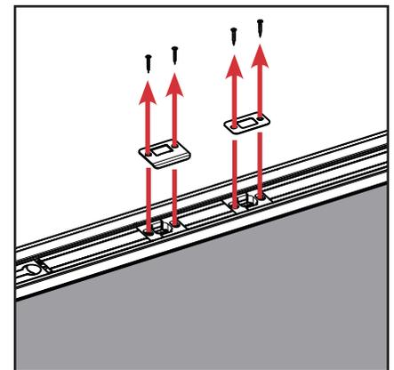
c. Once both retainers are in the astragal, screw on the strike plate and the deadbolt plate, using your best judgment for horizontal alignment.
