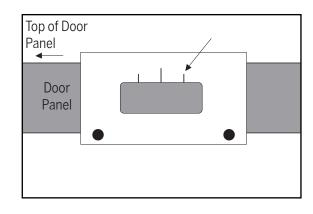
Line up the lower small mark on the router template with the location of the deadbolt centerline.
