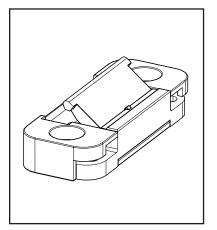
**NOTE:** Keeper pivot arm rests in upward position.
