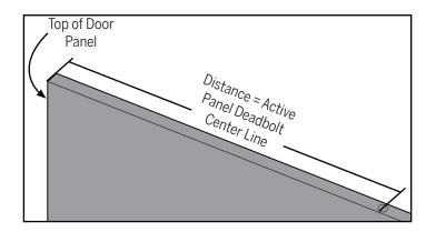
Mark the rout location on the inactive door panel.
