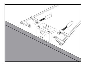
Position the bottom edge of the template slot 1/2" below the deadbolt center line.
