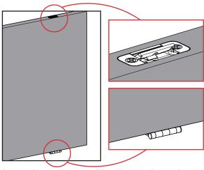
Insert keeper assembly into each pocket as shown. The open side of the keeper must face the the same side as the barrel of the hinges on the door panel.
