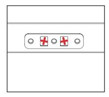
a. Using the marks you have made in Steps 1 and 2, line up the strike plate on the header.
