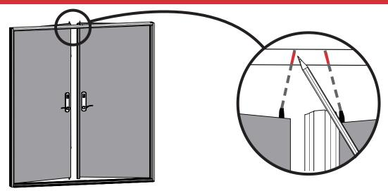
Close the inactive door and turn the lock to engage the upper and lower bolts. Mark the area where the lock will meet the header. This will serve as a reference point to mount the strike plate. Repeat this with the active door panel.
