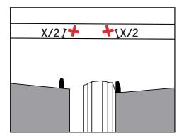
b. Divide this thickness (x) in half and mark the distance on the header. This will help you center the plate.
