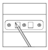
a. Trace the rectangular space of the strike plate with a pencil to use as a template to drill the holes.
