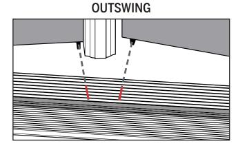
Close the inactive door and turn the lock to engage the upper and lower bolts. Mark where the lock meets the sill cap or deck. This will serve as a reference point to mount the strike plate. Repeat this for the active door.
