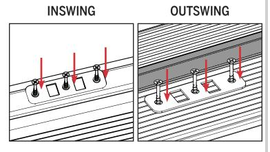
b. Spot drill the location of the screw holes. Once spot drilled, fully secure the plate into the sill with the screws provided.
