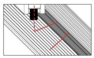
Close the door until the length of the door panel is parallel to the sill cap. Mark the centerline of the door panel onto the sill deck. Repeat for the other door panel.
