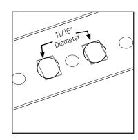
c. Drill into the header using an 11/16" diameter drill bit to create a space at least 1" deep.
