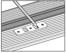
a. Trace the rectangular space of the strike plate to use as a template to drill the holes.
