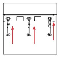
b. Spot drill the location of the screw holes. Once spot drilled, secure the plate into the header temporarily with the screws provided.
